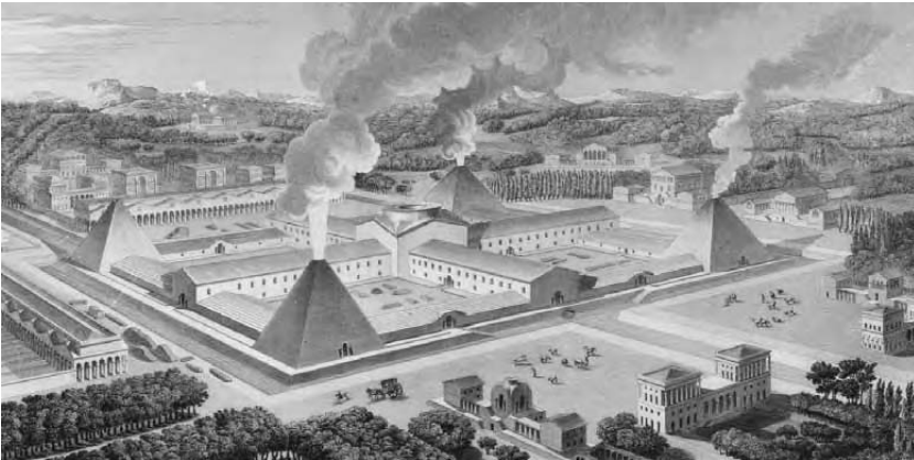
Plate 112 The Forge à Canons (planche 125) from C.-N. LEDOUX's L'architecture considérée , showing the use of pyramidal forms as corner-pavilions (in this case used as furnaces) (GN/SM).
